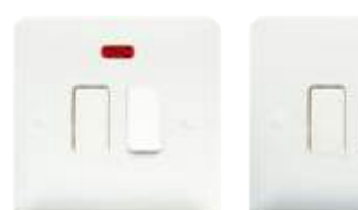
Z419 13A switched FCU'S + neon Z420 5A switched FCU'S + neon Z421 3A switched FCU'S + neon
