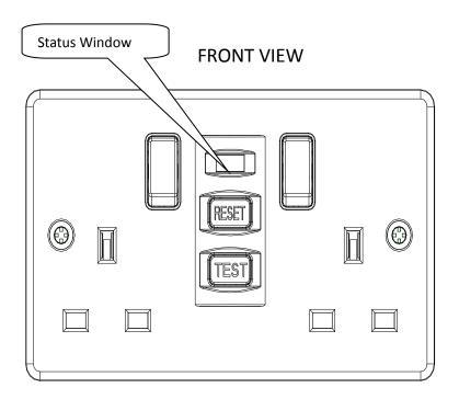
These devices with unique mechanical suspension means (latching pin) Closing the contacts will open automatically if there is an interruption in the mains supply.
