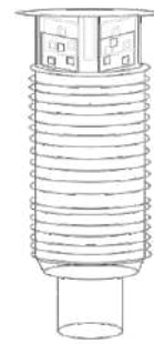
FZ-VL-001 Engineer pop up 4-side with 4*45 type outlets
