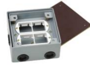
▲Temporary lid Secure to box body during concrete pour to prevent ingress of slurry. ▲Base box Ga-Steel box body:135x135x65mm
