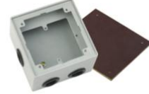
▲ Temporary lid Secure to box body during concrete pour to prevent ingress of slurry. ▲ Base box Ga-Steel box body:110x110x65mm
